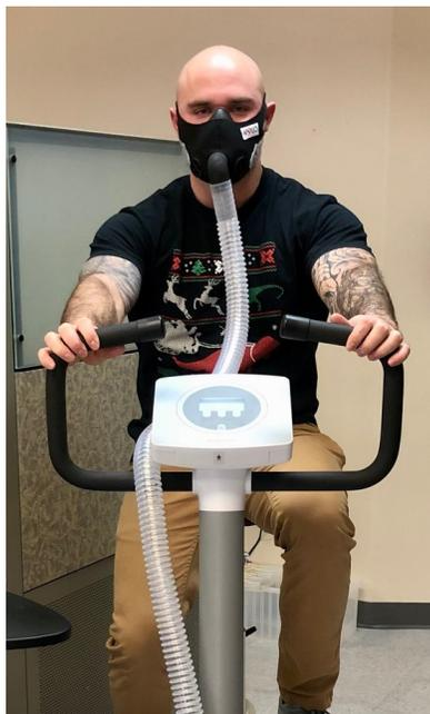
The Methane Analyzer can be coupled with the FMS indirect calorimetry system or the Promethion Room Calorimetry system for humans or when high resolution flow through measurements are required. The gas collection interface can be a mask, canopy, or custom enclosure.
