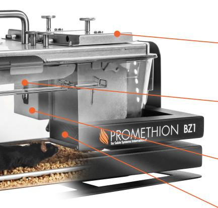
Fully Configured Respirometry Cage for Mice
